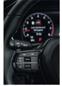
The sound system and various other features can be operated via the handy buttons on the steering wheel. Photos: Honda SA
