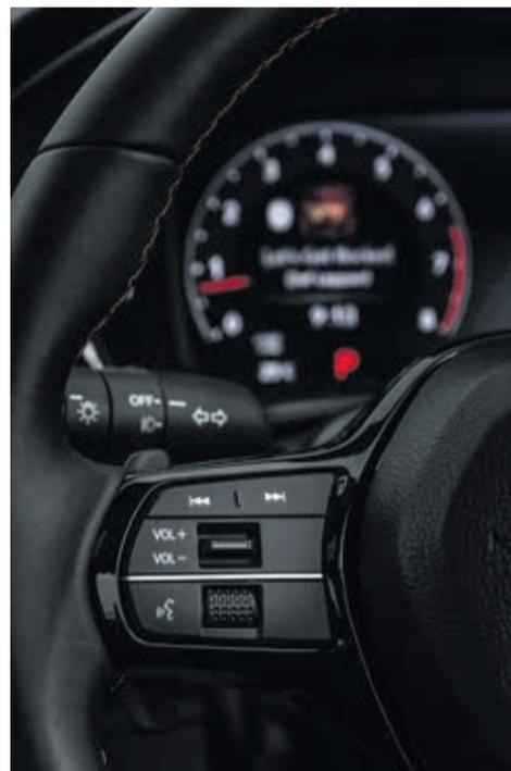
The sound system and various other features can be operated via the handy buttons on the steering wheel. Photos: Honda SA
